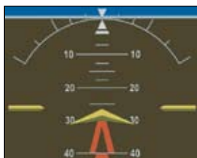
Figure 2-14 Extreme Pitch Indication
